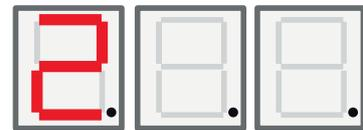
The relay display 2 has 7 sub items "201" – "207". The relay display will show the status of the relay as "On" or "Off".
